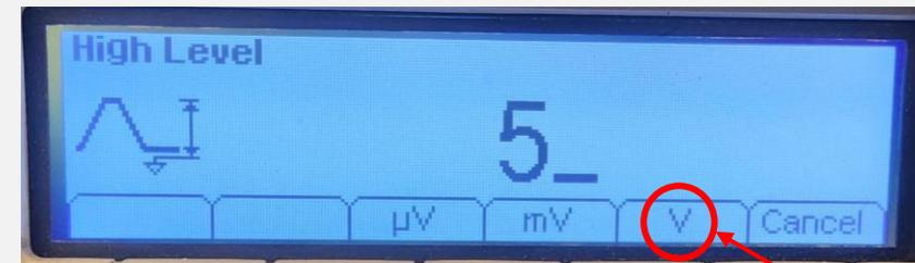
Press the button below *HiLev* (High Level) and it will display its current setting. Enter 5 using the number keypad and finalize your input by pressing the button below the appropriate scale in the newly displayed menu. For this exercise, select V (volts).
