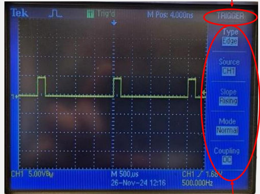
Press the Channel 1 button on your oscilloscope. This will display the Channel Menu on your screen as seen above. Make sure your settings match what is circled on the screen here. If not, cycle through the options by pressing the buttons alongside each menu item until it is identical.
