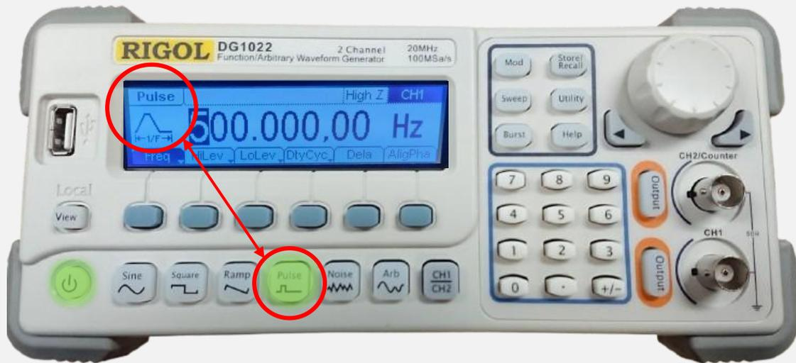
Change the type of waveform generated to a pulse. Pulses are ideal for measuring how systems respond to quick, temporary changes. You'll notice the waveform image and state shown in the display will change as well.
