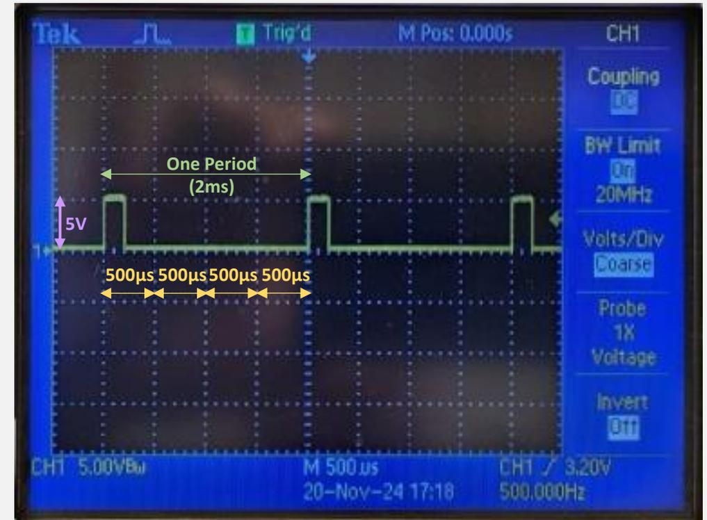
As you recall, we set our pulse generator to a period of 2ms (milliseconds) and a high level of 5 volts. Judging from the signal seen on our oscilloscope, we can see that everything is in working order. The amplitude is one box high, representing 5 volts, and the period, the length of time from the start of one pulse to the next, is 2000 microseconds which is equal to 2 milliseconds.
