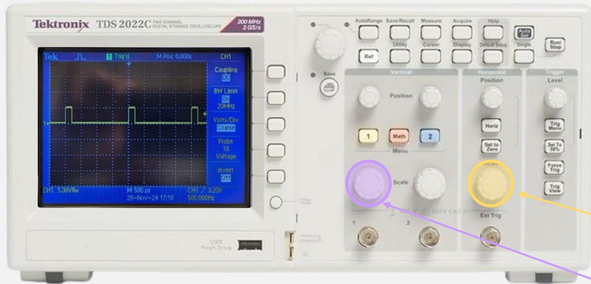
The knob highlighted in purple controls the voltage scale (y-axis). Adjusting this knob changes how much voltage each box in the grid represents. In this case, I have my scale set to 5 volts, so each box represents 5 volts.
