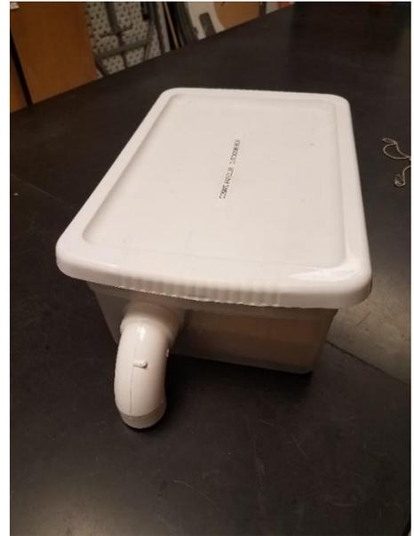
Place a 2" 90° PVC street elbow at the hole, and anchor it with a 2" male adapter on the inside of the box.
